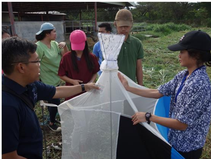
Tabanid trapping using the Nzi trap
